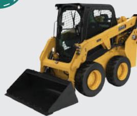
Skid steer loader Cat 232D
